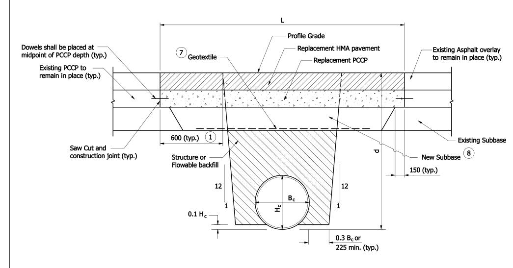
L = Pay limits of pavement removal and pavement replacement (m); for cross pipe, measured along roadway centerline; for pipe parallel to roadway centerline, measured prependicular to pipe centerline.
