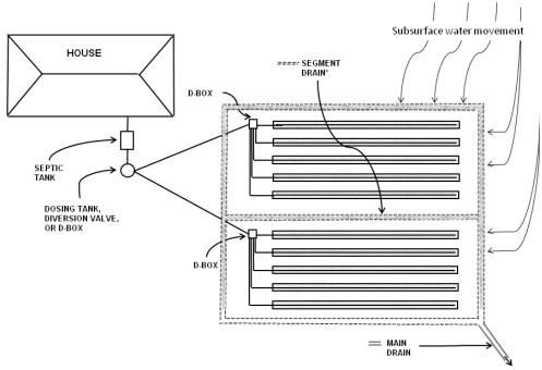
\*The segment drain may be backfilled with aggregate. The upslope drain backfilled with aggregate may need to extend down the ends of the soil absorption field trenches to intercept and divert all subsurface water. Aggregate may also be used in the downslope drain.
