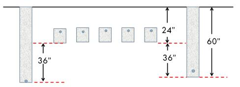
Figure 6: Perimeter Drain Depth for a SAF on a Sloping Site
