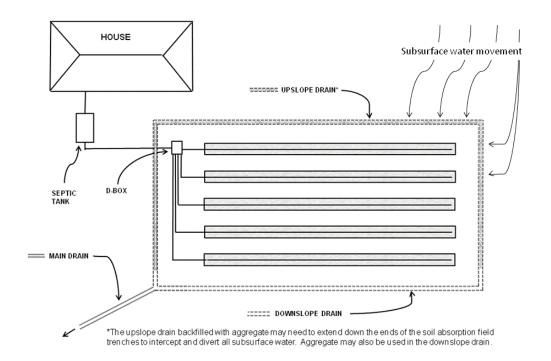
Figure 3: Subsurface Interceptor Drain on a Sloping Site
