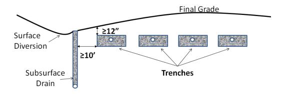
Figure 2: Subsurface Perimeter Drain on a Sloping Site
