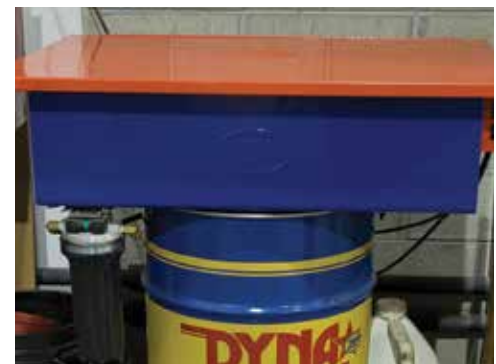
Properly closed parts washer.
