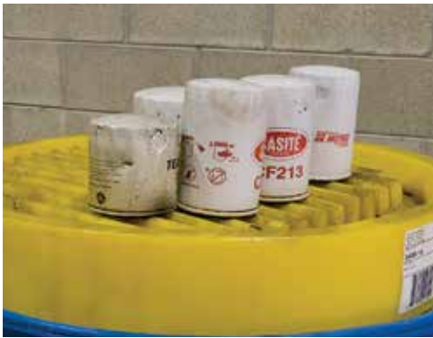
Oil removed and drained from oil filters.
