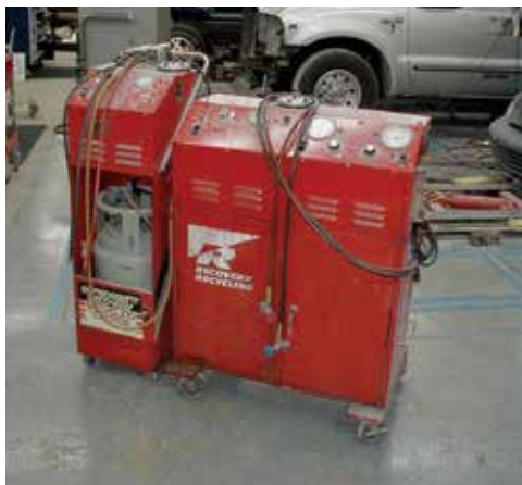
Refrigerant recovery device.
