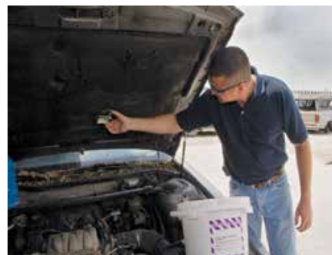
Removal of mercury switches is required by Indiana law.
