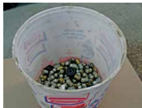
Improper mercury switch storage.
