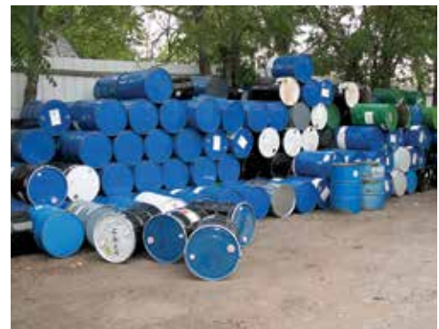
Drums capped and stored on their sides.
