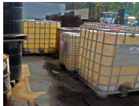
Oil storage capacity exceeding 1320 gallons.
