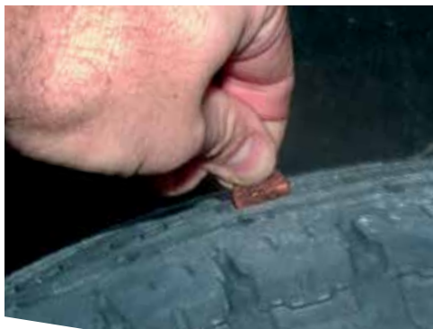
2/32 inch tread depth test with a penny.
