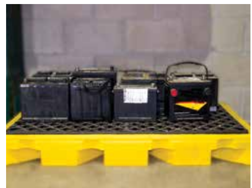
Batteries stored inside with secondary containment.
