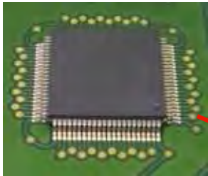
QFP: no fails @ 5500 cycles SnPb or Pb Free
