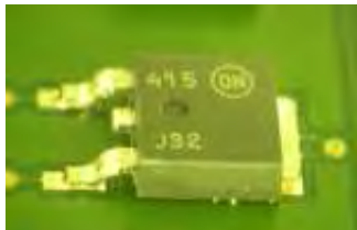
DPAK: no fails @ 5500 cycles SnPb or Pb Free
