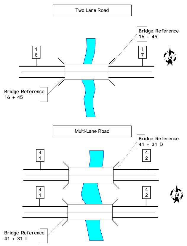
Figure 16: Detail Bridge Referencing
