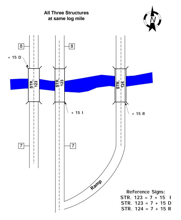
**Figure 18: Detail Multiple Structures Same Location**
