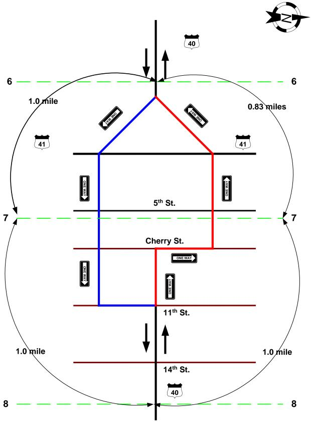
**Figure 13: Detail of One - Way pair** Revised May 1999
