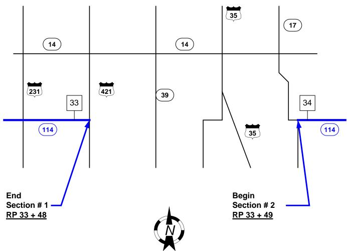
**Figure 14: Detail Discontinuous Routes**
