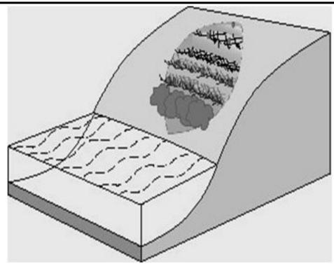
Branch packing quickly establishes a vegetated bank to prevent runoff and contain erosion. The branches trap sediment while the roots stabilize and dry out the soil. As the vegetation grows, efficiency increases because plant leaves reduce soil runoff that can result from the impact of rain.
