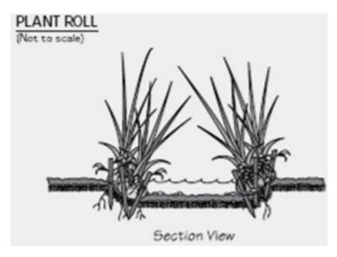
Ideal places for plant rolls are in areas where rapid repair of minor damage is needed. Many native species can grow in a plant roll, including many species of sedges, rushes, and grasses. Rolls are ideal where these types of plants normally grow. Unlike seeding, plant rolls can withstand areas of fluctuating water. Because rolls collect sediment and improve the microclimate, native species can easily become established and survive around a roll. Rolls offer immediate toe protection.
