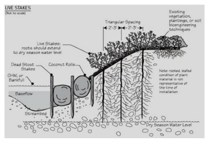
Live stakes can be installed in conjunction with other bioengineering materials, such as geotextile fabric, coconut fiber logs, and live fascines. If a streambank is exceptionally prone to erosion, laying geotextile with the live stakes helps control erosion while the live stakes take root. Live posts are quite similar to live stakes, only live posts are much larger (USDA 2002).
