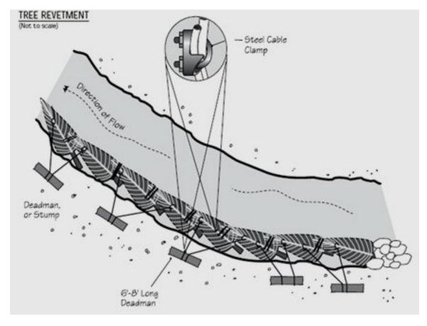
Log, root wad, and boulder revetments are a combination of bioengineered materials using the ideas from log revetments and boulder revetments. This technique is often used when added erosion protection is needed (USDA 2002).
