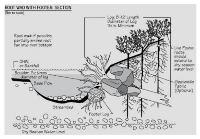
Most root wads are quite large and require heavy machinery for installation, which can cause increased stream sedimentation (Alaska Department of Fish and Game 2005). Use is also site limited. If undercutting is likely, root wads should not be used. Also, they cannot be used in braided streams or with sandy or silty soil. Regular
