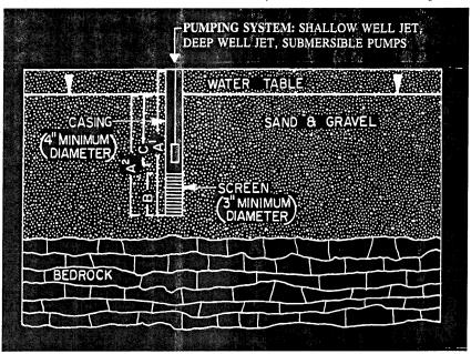
A<sup>1</sup>) Well shall be a minimum of 30 feet in depth.
