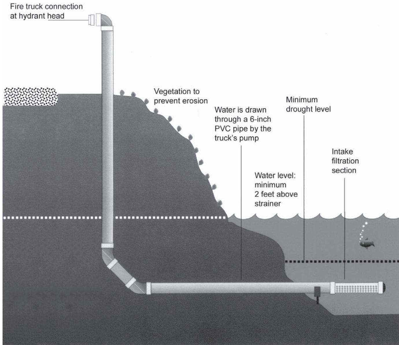
A dry fire hydrant is simple in design, but provides improved fire protection and lower insurance rates to you and your neighbors. It must be installed on a road that provides easy fire truck access.
