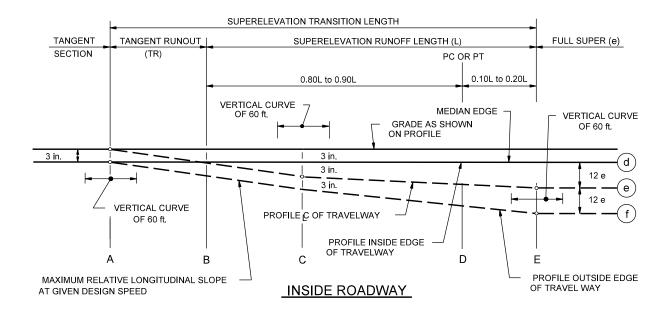
NOTES: 1. AXES OF ROTATION ABOUT TWO MEDIAN EDGES 2. e = APPLICABLE SUPERELEVATION RATE
