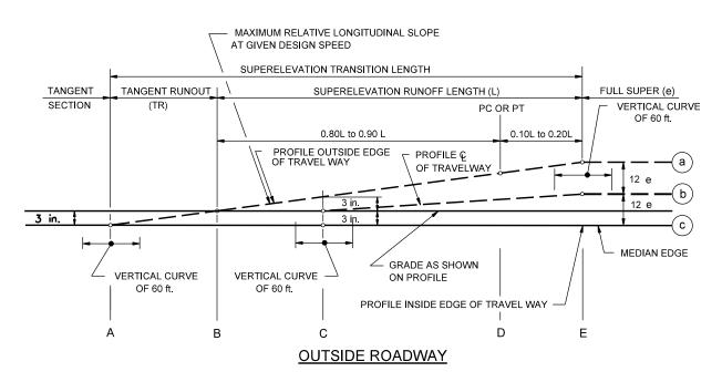
NOTES: 1. AXES OF ROTATION ABOUT TWO MEDIAN EDGES 2. e = APPLICABLE SUPERELEVATION RATE
