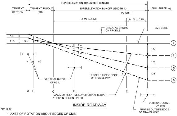
1. AXES OF ROTATION ABOUT EDGES OF CMB 2. e = APPLICABLE SUPERELEVATION RATE
