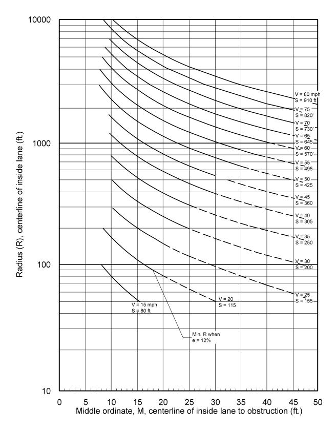
DESIGN CONTROLS FOR STOPPING SIGHT DISTANCE ON HORIZONTAL CURVE
