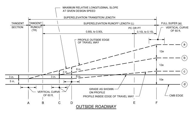
NOTES: 1. AXES OF ROTATION ABOUT EDGES OF CMB 2. e = APPLICABLE SUPERELEVATION RATE
