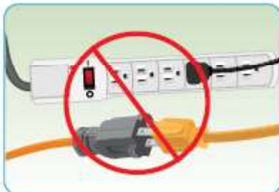
Do not use extension cords or power strips with an ON/OFF switch.
