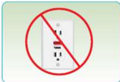
Do not use outlets that have built-in circuit switches (they have red reset buttons).
