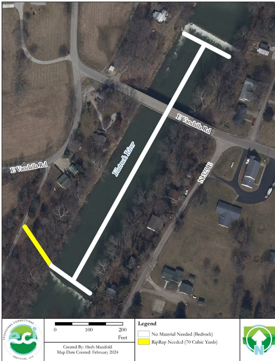
Figure 14. Equipment path needed to access Flatrock River (Geneva) dam. This pathway is already clear large woody vegetation as it is a mowed lawn. White sections of the pathway will require no additional material for access. Yellow sections of pathway will be used as a footing for the removal equipment, A maximum of 70 cubic yards of riprap will be utilized. All material will be removed when the project is complete.
