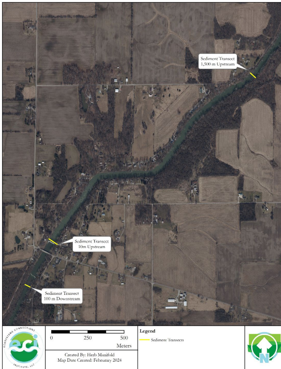
Figure 4. Site of each of three transects for collection of sediment samples. Sediment samples were collected at 25%, 50%, and 75% of the stream width at each of the three transects. Transect one is 100-meters below the most downstream dam, transect 2 is 10-meters above the most upstream dam and transect three is 1.5 km upstream of the most upstream dam.
