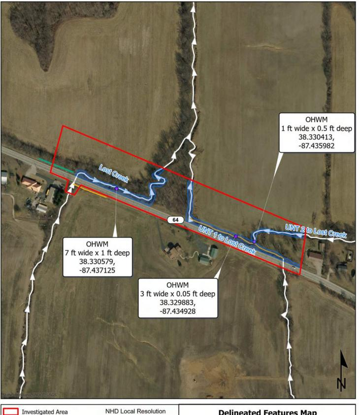
NHD Local Resolution **Delineated Features Map** Canal/Ditch SR 64, 2.3 Miles West of I-69 **Delineated Stream** Slide Correction Stream/River **OHWM Point** Gibson County, Indiana RSD #1 Des. No. 2100263 125 250 0 1 inch = 250 ft Feet Graphics created by HNTB Corporation (2023)
