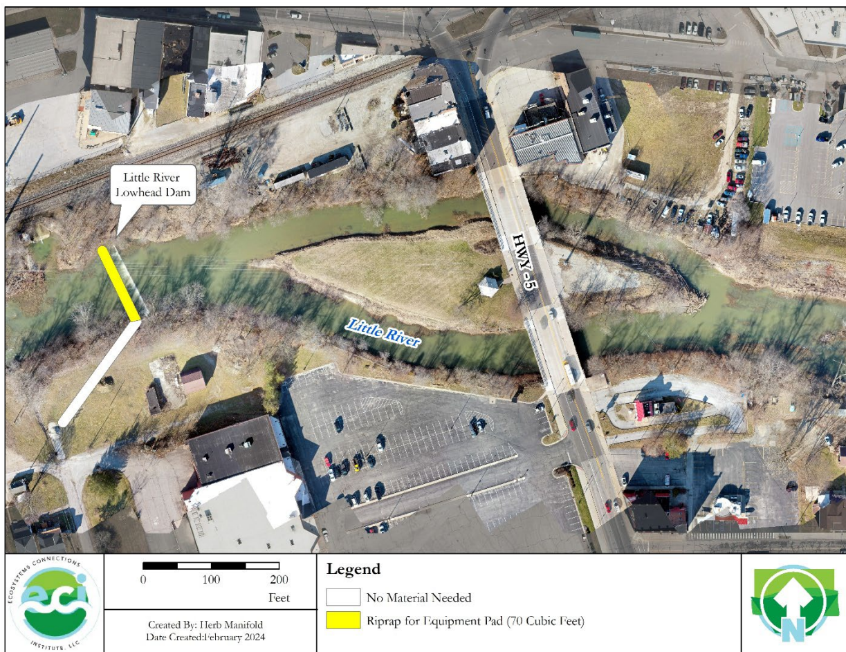
Figure 6. Equipment path needed to access Huntington dam. This pathway is already clear large woody vegetation as it is a mowed lawn. White sections of pathway will require no additional material for access. Yellow sections of pathway will be used as a footing for the removal equipment, A maximum of 70 cubic yards of riprap will be utilized. All material will be removed when the project is complete.
