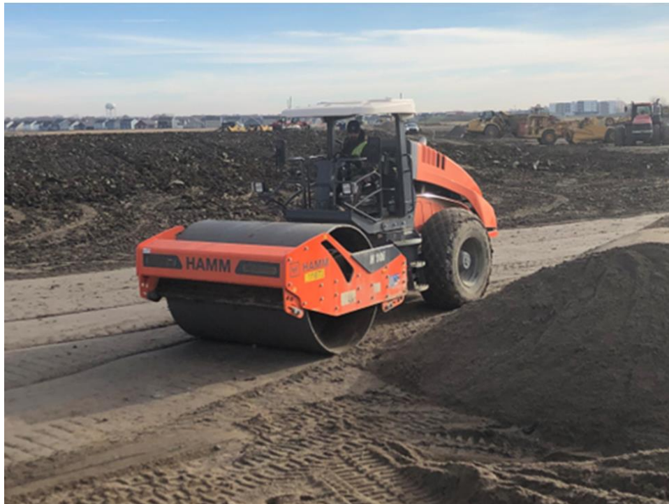
Figure 58. Typical steel, smooth-drum vibratory roller for compacting backfill outside of 3 ft from pre-cast panels
