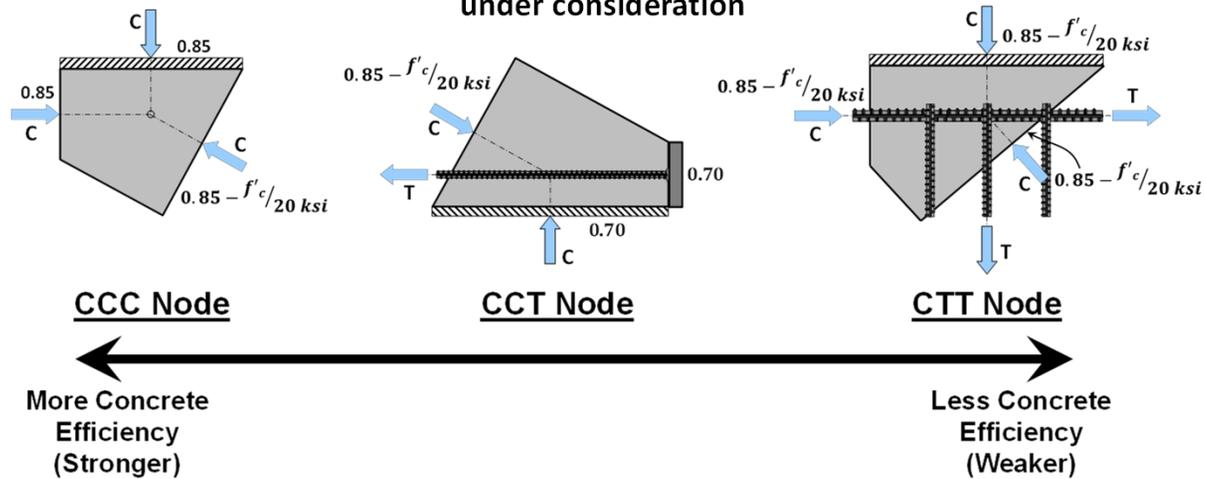
***If the web crack control reinforcement requirement is not satisfied, use  $v = 0.45$  for the strut-to-node interface***
