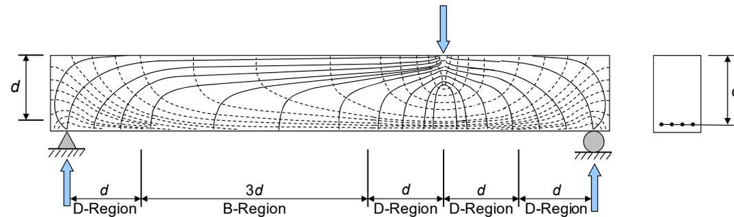
Figure: Stress trajectories within structural member
