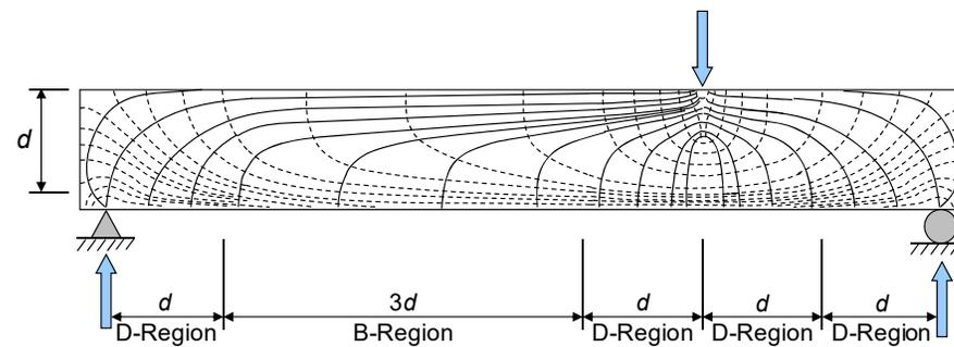
Figure: Stress trajectories within structural member
