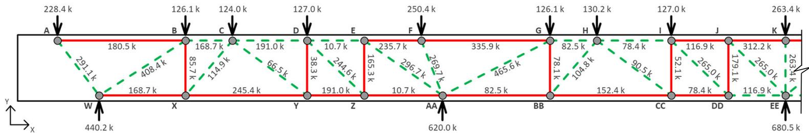
**Performs Strength Checks and Other STM Design Procedures**
