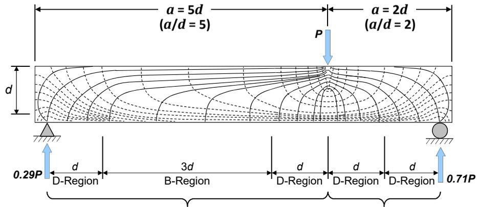
Shear-span-to-depth ratio  $\longrightarrow$
