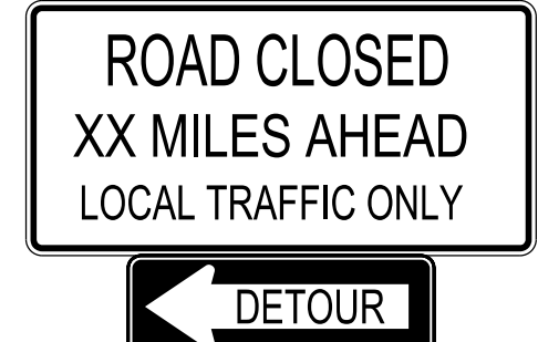
ROAD CLOSED XX MILES AHEAD LOCAL TRAFFIC ONLY XM4-10 (R or L) R11-3 16
