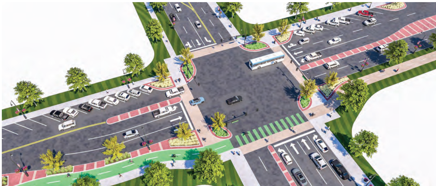
Creative solutions to barriers: A protected intersection in Downtown Olathe, Kansas. The cycle track portion is in the process of development.
