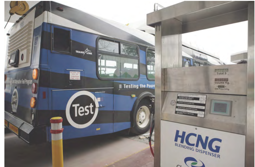
Natural gas dispenser for Canadian bus fleet. Photo from hydrogenhighway.ca .
